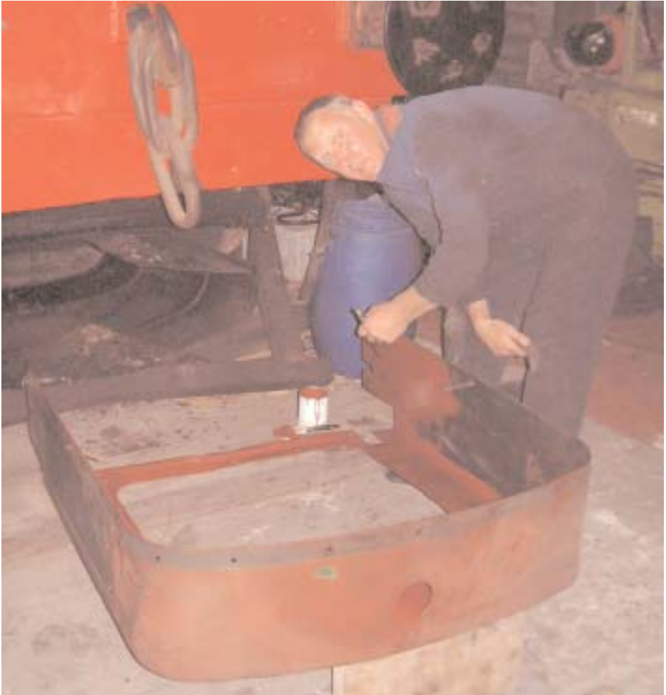
Baz Shell looking startled during application of a coat of red oxide primer to the ruston cowling. Photo: M. Murray
